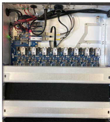
(a) A daisy chain of 8 Irises assembled within an enclosure. Part of the daisy chain is hiding under a heat sink. The Irises connect to the hub through a power and fiber cable.
