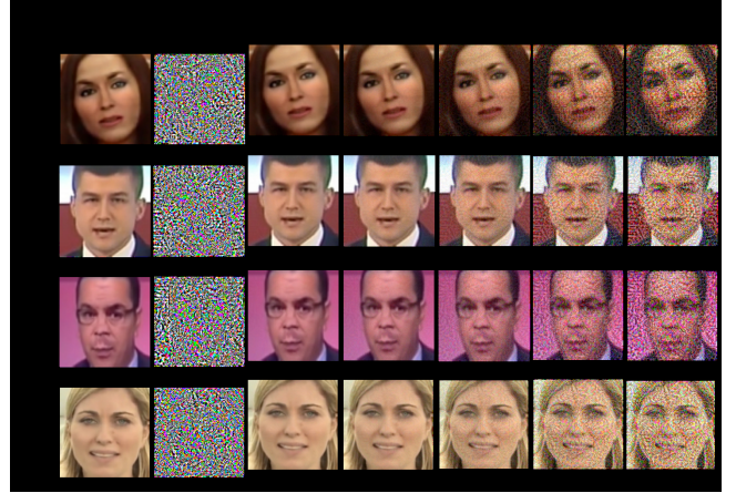
Figure 4: Adversarially perturbed frames extracted from randomly selected deepfakes from the FaceForensics++ test set. The input frames are classified as Fake by the victim models. The perturbed frames generated according to different \epsilon values using FGSM are shown in each row. Perturbed frames whose \epsilon > 0.01 are labeled as Real by the victim models. The distortion increases proportionally with \epsilon .
