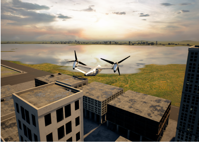
Fig. 3. Tiltrotor eVTOL vehicle flying in AirSim simulation environment using our ROS2 trajectory tracker and altered PX4 Autopilot Software.
