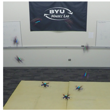
Fig. 1. Time lapse image of our proposed geometric control scheme tracking a flipping loop trajectory.
