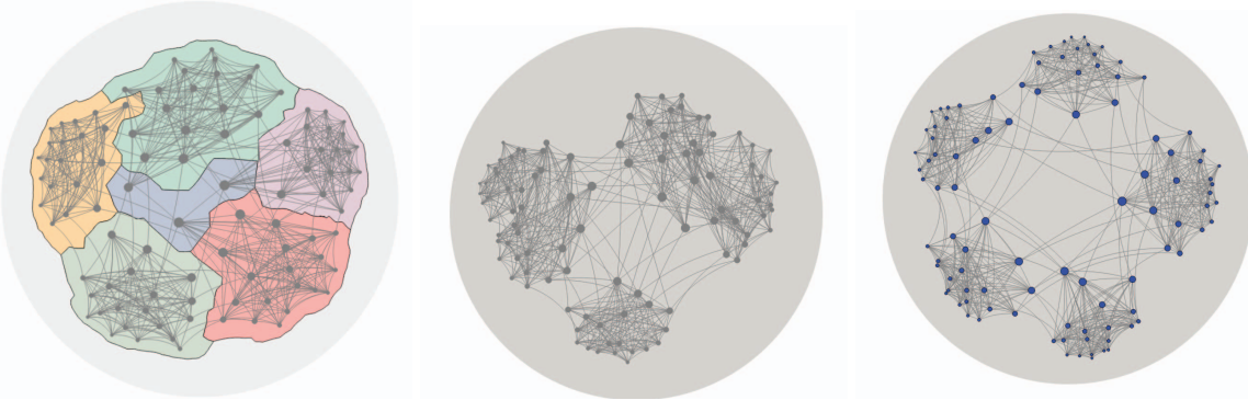
Figure 1: Example layouts of the same graph, generated by the three hyperbolic graph embedding algorithms discussed in this paper: inverse projection (left), force-directed (center) and hyperbolic-MDS (right).
