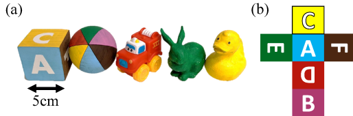
Fig. 6. (a) We experimentally validate our method with 5 different objects, namely a cube, sphere, toy truck, Stanford Bunny, and toy duck. (b) Tessellated faces of the cube show poses of the affixed letters.
