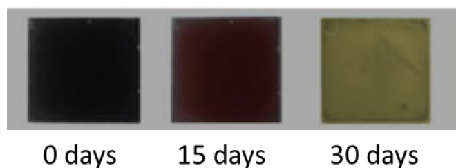
FIG. 4. Degradation of MAPbI 3 film (left, black) to PbI 2 (right, yellow) over 30 days stored in air at 50% RH. Reprinted from reference [54], with permission. Copyright 2019, John Wiley and Sons.
