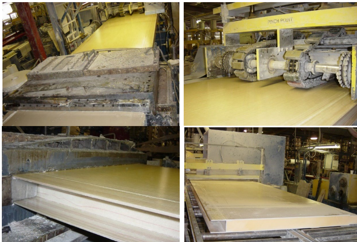
Fig. 1. Pultrusion of 4' wide GFRP panels at BRP
