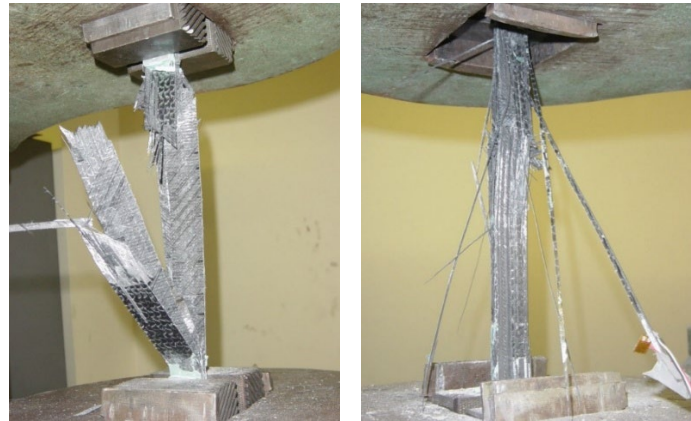
Fig. 10. Typical failed tension specimens for carbon /VE (left) vs. carbon/epoxy (right)
