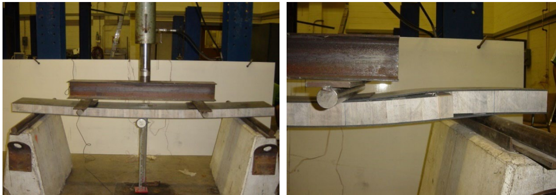
Fig. 15. Four point bending with a span of 80'' for 12'' x 96'' CFRP panel
