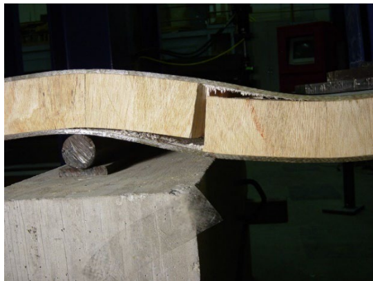
Fig. 7. 3.5" VARTM panel (5' x 5', provided by NSWC) being tested to failure with exposed cracking
