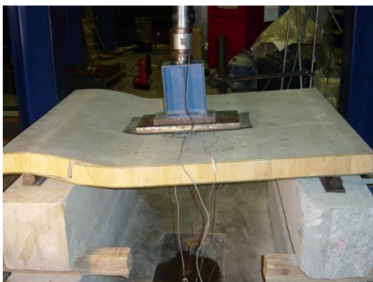
Fig. 7. 3.5" VARTM panel (5' x 5', provided by NSWC) being tested to failure with exposed cracking
