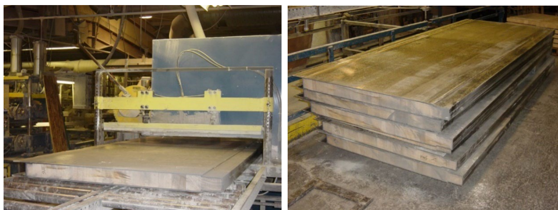
Fig. 3. Pultrusion of 4' wide CFRP panels at BRP
