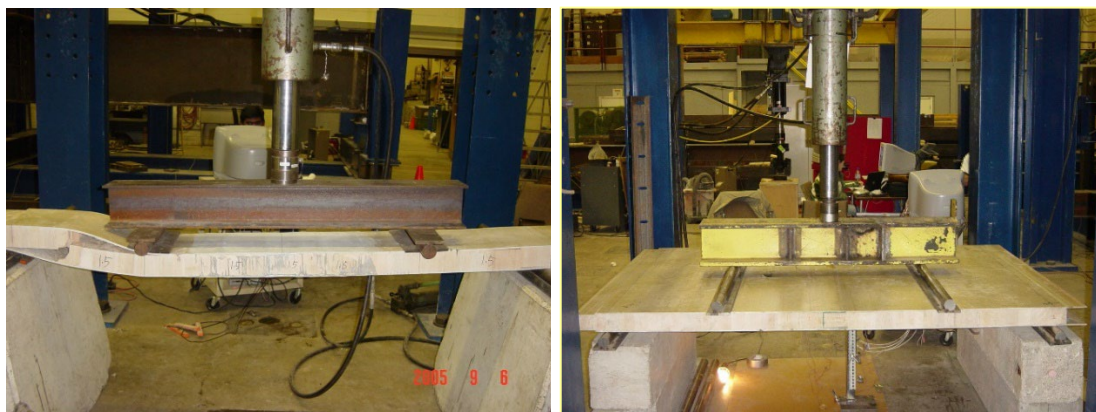
Fig. 16. Joined panels (left, 12' x 96'; right, 5' x 8') of 100% joint efficiency under 4 pt bending
