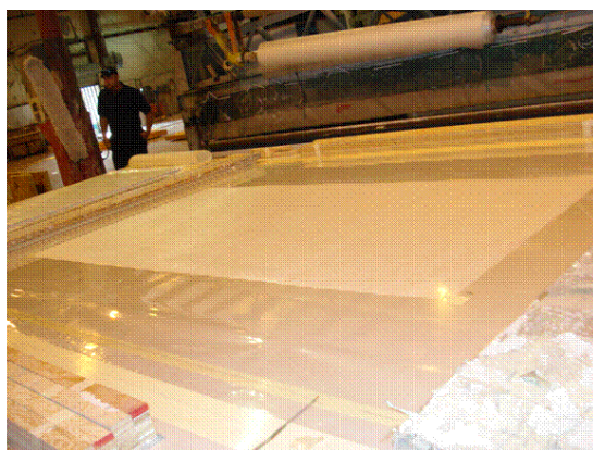
1) Placement of fabric
