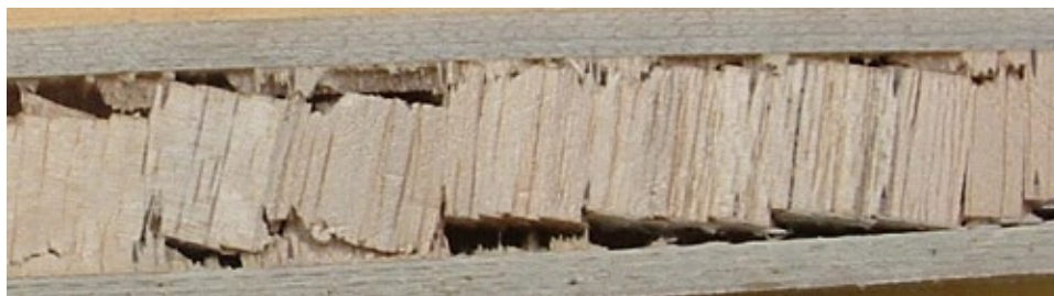
Fig. 2. A cohesive bending failure of sandwich panel showing good bond between balsa and FRP skin
