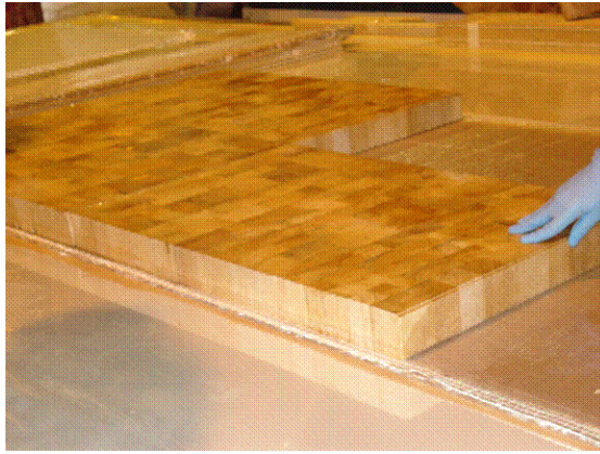
3) Placement of core panel
