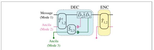
Figure 5. General architecture of CV QEC protocol. The light blue shaded area denotes decoding (i.e. DEC), and the light yellow shaded area denotes encoding (i.e. ENC).
