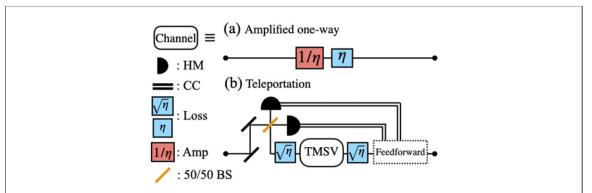
**Figure 2.** The scheme of (a) amplified one-way channel, and (b) teleportation channel. CC: classical communication. HM: homodyne measurement. Amp: amplification. BS: beamsplitter.
