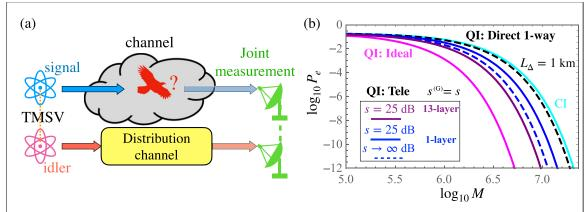
**Figure 11.** (a) Scheme of quantum illumination. (b) The quantum Chernoff bounds of error probability  $P_e$  versus transmitted M modes for CI and three QI cases: ideal entanglement distribution, direct one-way, and m-relay k-layer (k = 1, 13) QEC with teleportation at L = 25 km with  $N_S = 0.01$ .
