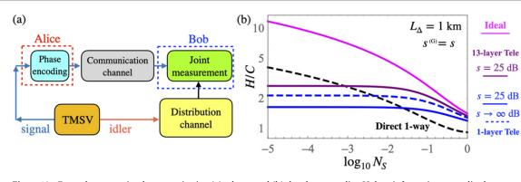
**Figure 10.** Entanglement-assisted communication (a) scheme and (b) the phase encoding Holevo information normalized to classical capacity (H/C) at L=25 km for the cases of ideal, direct one-way transmission and m-relay k-layer (k=1,13) QEC with teleportation.
