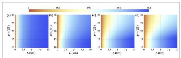
**Figure 7.** Fidelities of teleportation-based QEC QR based on imperfect GKP. Input TMSV is set r=15 dB and the inter-repeater separation is  $L_{\Delta}=1$  km. (a) s=10 dB ( $L_{\Delta}^*=4.6$  km), (b) s=15 dB ( $L_{\Delta}^*=1.4$  km), (c) s=20 dB ( $L_{\Delta}^*=0.44$  km), (d) s=25 dB ( $L_{\Delta}^*=0.14$  km).
