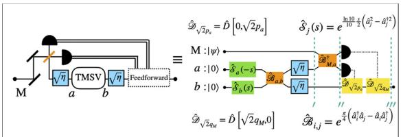
**Figure A1.** The quantum circuit scheme of teleportation. The apostrophes, ', " and "', stand for the stages, mentioned in the context.  $q_M = \langle \hat{q}_M^{(\Gamma)''} \rangle$  and  $p_a = \langle \hat{p}_a^{(\Gamma)''} \rangle$ .
