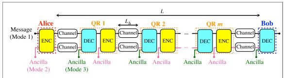
**Figure 1.** Scheme of m-relay repeaters based on CV error-correction protocol. ENC: encoding. DEC: decoding. L is the physical distance between Alice and Bob.  $L_{\Delta}$  is the inter-repeater spacing.
