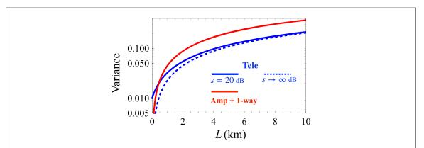
**Figure 3.** Variances of the additive noise for the protocols of amplified one-way and teleportation channels. Amp: amplification. Tele: teleportation.
