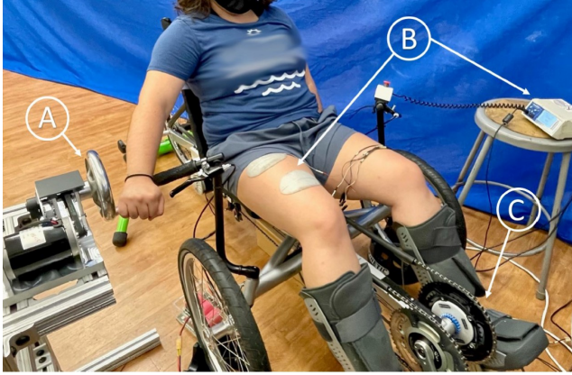
Figure 1. A teleoperated cycling testbed is shown, where A denotes the leader (hand-cycle), B denotes the FES unit and corresponding stimulation pads placed on the right quadriceps, and C denotes the follower split-crank cycle.
