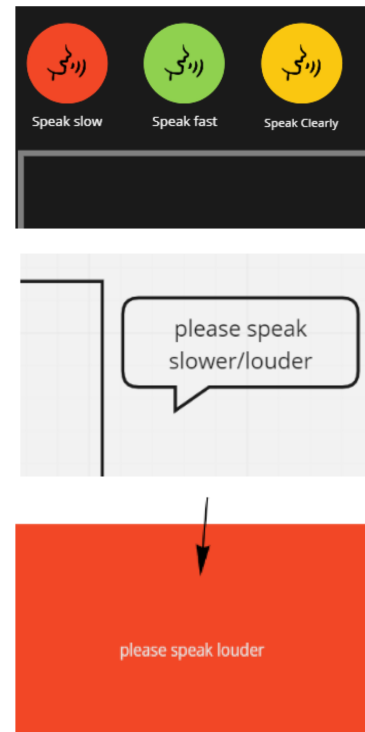
Figure 7: Three distinct notification styles resulted from our workshops: (a) Icons (pictured top) that persist on the screen and enlarge to notify the speaker to speak slow, speak fast, or speak clearly. (b) A pop-up bubble (pictured center) next to the speaker’s video with text-based notification. (c) A screen overlay (pictured bottom) atop the speaker’s entire video with text instructions to speak louder.
