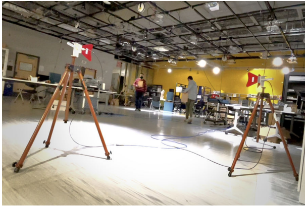
(a) Sub-6 GHz SDR Radar for MTT with Two Copper Plates
