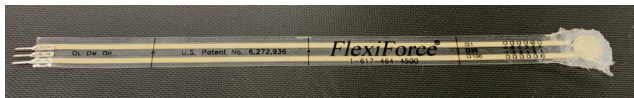
Fig. 6. The silicone coated Flexiforce Standard Model A201 FSR used for testing grasping force.
