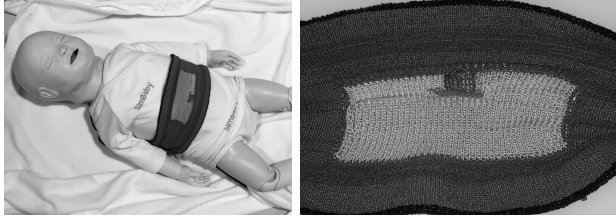
Fig. 1: Left: the Bellyband on an animatronic mannequin called a SimBaby [5]. Right: close up of the antenna portion of the Bellyband. Note the darker non-conductive material, the lighter conductive thread antenna, and the grey square inlaid in the lighter thread, which is a non-conductive pouch housing an RFID chip and matching circuit.
