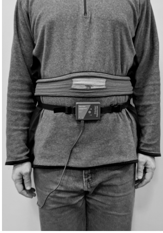
Fig. 7: Bellyband and Vernier Go Direct Respiration Belt on subject. The Respiration Belt (below), a wired sensor, was used to verify ground truth respiratory rate. The datastreams from the sensors were synchronized by the subject taking a particularly deep breath at the beginning and ending of the data collection - creating a noticeable wave signature in both streams.
