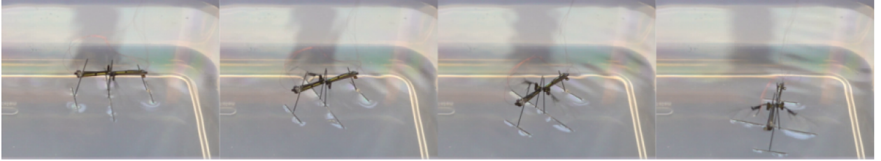
Fig. 20. RoboFly performing water surface locomotion and turning left with open loop control by flapping wings at 30 Hz, frames are captured at 0, 1, 2, and 3 s
