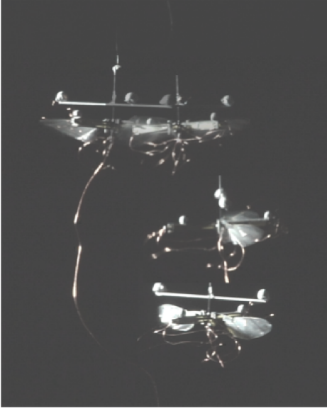
Fig. 13. Flight in which the robot takes off and hovers about a reference point in space with the help of feedback from a motion capture arena. The robot is subject to a small yaw bias torque that caused it to rotate leftward in this video [38].
