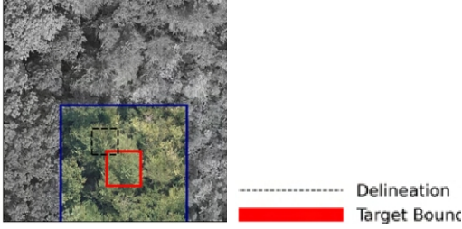
Fig. 3. An example of issues with missed delineations and inappropriate parameters. An example of a missed delineation that has an inappropriately high RC value ( RC = 0.99 , IoU = 0.02 ) given parameters that resulted in zero variance between annotators. The zero variance parameters are: true positive boundary 10 cm, true negative inner boundary 30 cm, and area ratio 7. The same delineation with our selected parameters; true positive boundary 70 cm, true negative inner boundary 1.2 m, and area ratio 3 scores a zero as a missed delineation ( RC = 0 , IoU = 0.02 ). As the true negative inner boundary parameter is too large with a slightly larger area ratio, all scores are near one even in cases where the delineations clearly do not match the desired target. It is possible that the high RandCrowns measure could be negated by reducing the area of the true positive boundary. However, that would merely fix this type of missed delineation and not necessarily be applicable for other delineations that would encompass small parts of the true positive boundary and much larger areas of an immense false region.
