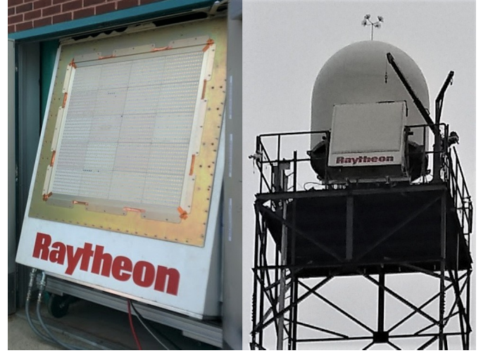
Fig. 3. (Left) View of the radiating face of the Skyler Radar prototype with the radome removed. (Right) Photograph of the Skyler Radar installed on the Orchard Hill Tower on UMass Campus.
