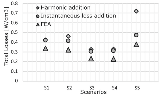
Fig. 8. Average total losses in a single filament conductor in \text{W}/\text{cm}^3 at 10 Hz.
