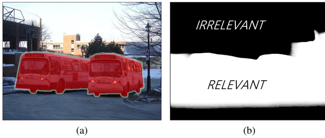
Figure 1: Example of irrelevant pixels in a PASCAL VOC dataset image. (a) The shuttle buses are highlighted in red. (b) Our method shows that a significant number of pixels (black) are irrelevant, providing little utility, even though CNNs waste computation on them.
