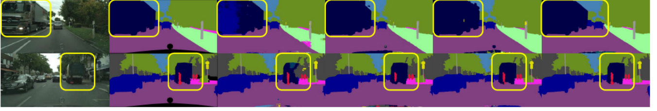
Fig. 9. Some visual examples of segmenting outputs on Cityscapes validation set, when boundary cues are sequentially introduced. From left to right are input image, Ground truth, segmentation results using backbone, backbone + SFB, backbone + SFB + BFB(without VS), and backbone + SFB + BFB (with VS). Dilated-ResNet101 is used as backbone. (Best viewed in color.)
