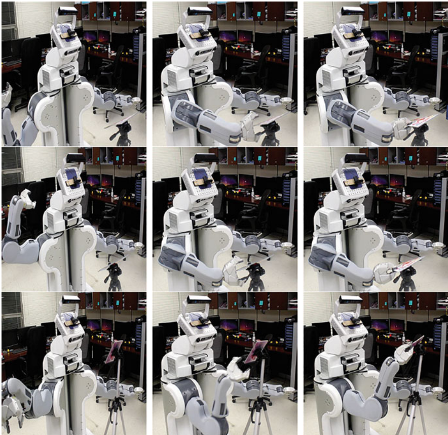
Fig. 11 Robot grasping an object from a tripod. Left: initial position of the robot's gripper, middle: gripper adapting to the object's pose, right: grasping of the object
