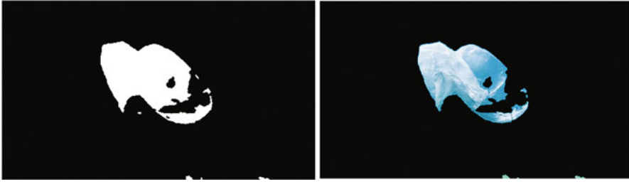
Fig. 9 (Left) Improved debris mask after morphological operations. (Right) Identifying single large piece of debris object using the binary mask
