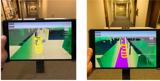
Fig. 8 Two examples of AR immersive views on iPad, taken from different locations in a building. The right one also shows the navigation path in purple.
