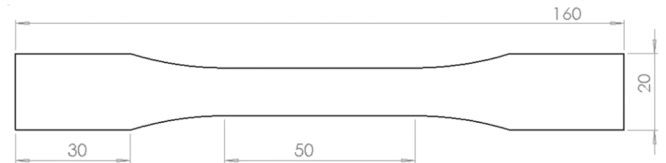
Fig. 1. ASTM E8 uniaxial tension specimen and dimensions in millimeters.
