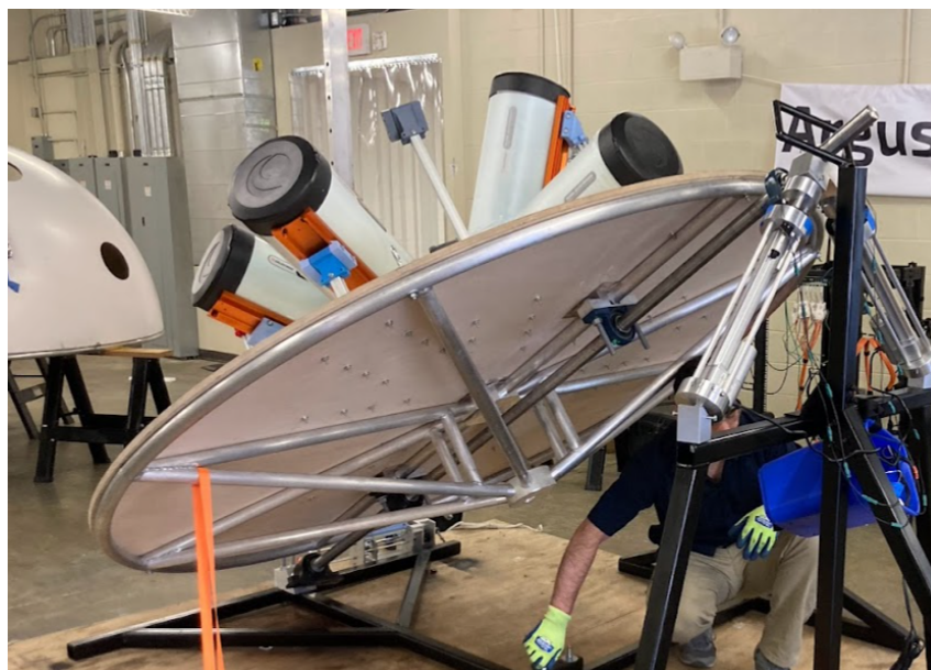
Figure 2. Telescope support platform, installed on the low-cost “Hercules” mount structure, during lab integration testing.
