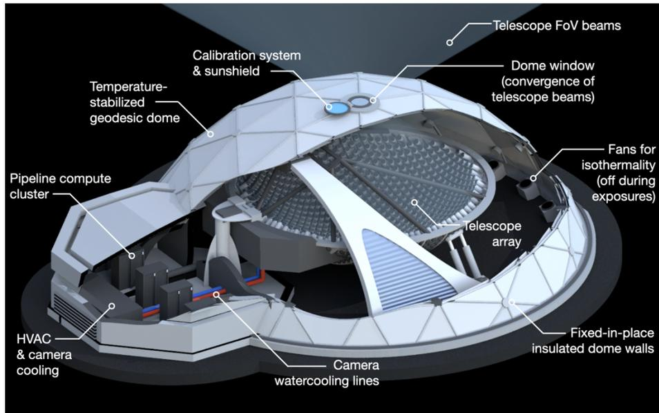
Figure 1: Model of the Argus Optical Array in its  $\approx 60$ -foot diameter enclosure. With over 900 8-inch aperture telescopes sharing a single mount and enclosure, the Argus Optical Array will have the etendue of a 5-m-class telescope and image 20% of the sky instantaneously. Thousands of moving parts and optical elements are protected within a stable environment.<sup>3</sup>
