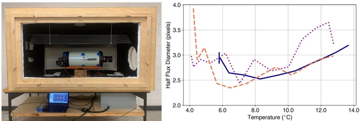
Figure 4: *Left:* The Delta-T Test Enclosure. A Celestron RASA-8 with a QHY600 camera is shown mounted on a block and centered on the round viewing window (right). The temperature is recorded with 11 RTD sensors distributed uniformly over the telescope body (covered in blue tape). The enclosure can be tilted to point at the NCP.
