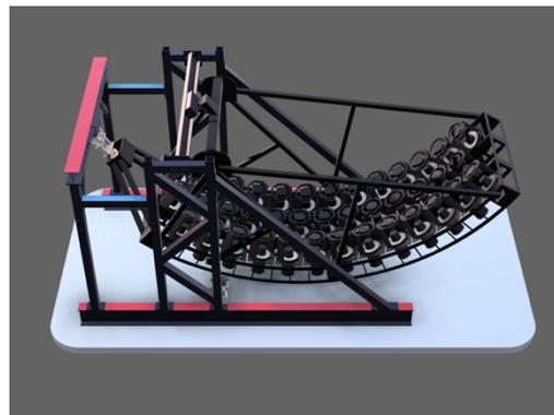
Figure 2: *Left:* The Pathfinder mount under construction with team members (left to right): Alan Vasquez Soto, Jon Carney, Hank Corbett. The array will fit inside a 20-foot shipping container with a separate container for support equipment. *Right:* Model of the completed Pathfinder array structure. Thirty-eight Argus-8 telescopes are mounted on a curved “cradle” and observe a segment,  $92^\circ$  long in declination, of the full Argus Array field of view.
