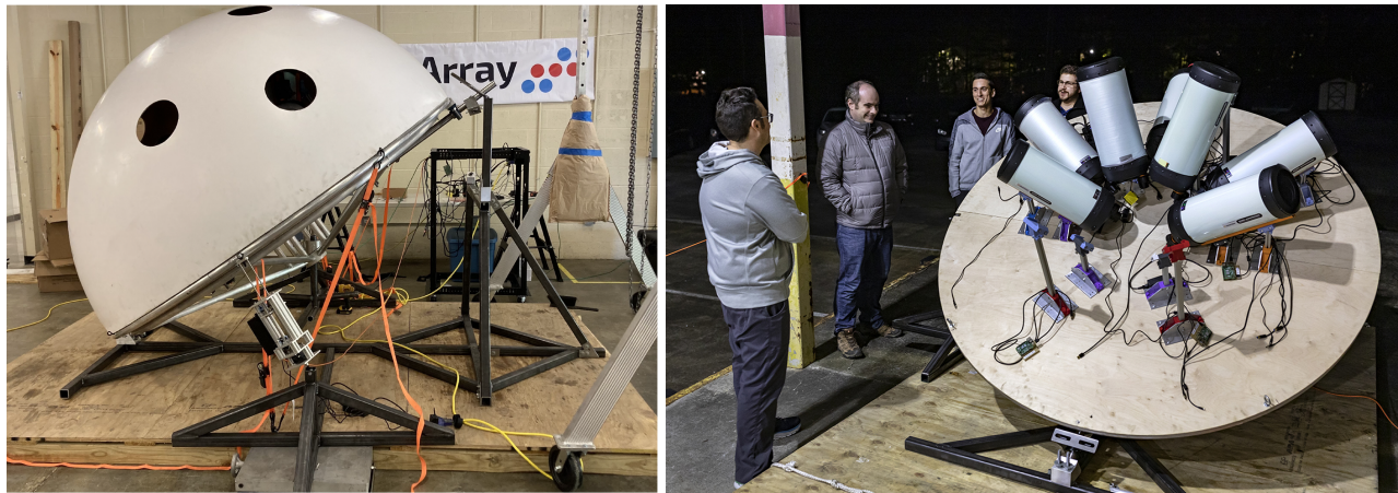
Figure 5: Left: The fully constructed Hercules Mount with the dome installed. Right: The A2TD with the dome removed showing the telescope mounting configuration on top of the telescope platform. ( Image credit: Johnny Andrews/UNC-Chapel Hill )
