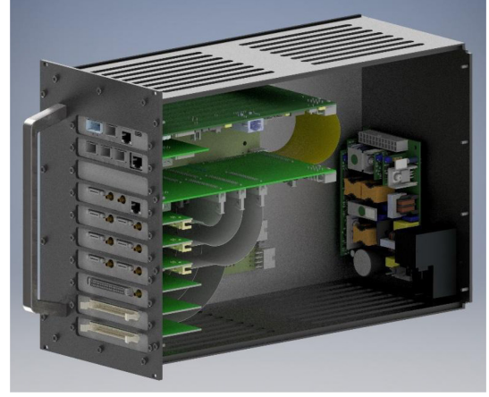
Figure 5: Rack (left) including the interface module and high voltage control boards; and rendering of boards (right) internal to the interface module.
