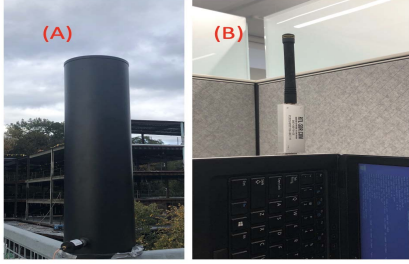
Figure 8: Hardware used in SelfieStick (A) Weather Antenna, (B) RTL SDR with Laird Antenna
