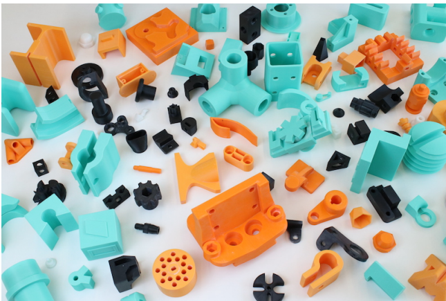
Fig. 8. A photo of the thermoplastic 3D CAD models fabricated for the evaluation of our approach in a real-world setting.
