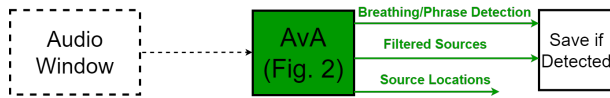
Figure 4: AvA-enhanced platform for filtering out speech and preserving privacy in mobile applications. Unlike in urban safety, audio privacy applications save raw breathing sounds. In the AvA-enhanced systems, we save the filtered signals rather than the raw audio to preserve privacy.
