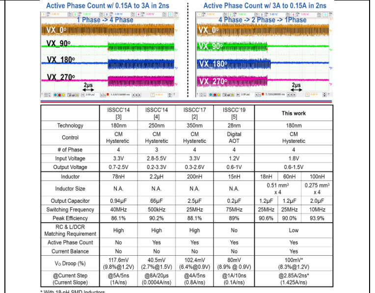
Fig. 6. Measured V_X with APC operation, and comparison table.
