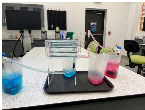
Figure 2. Double pipe set up
