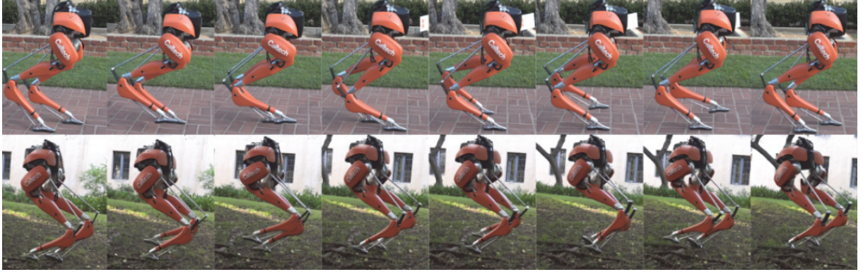
Fig. 8. Gait tiles of the robotic walking exhibited experimentally on the Caltech Cassie robot. The top half is two steps of flat-ground forward walking outside, while the bottom half shows several steps of the robot walking over a height variation caused by both a shallow grassy slope and exposed roots.
