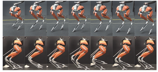
(b) The robustness (top) and tracking (bottom) of the walking with the learned optimal gains, enabling unassisted, stable walking and good tracking performance.
