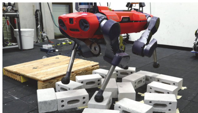
Fig. 1. ANYmal [6] performing a trotting gait on stepping-stones.
