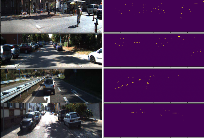
Fig. 8. Outliers with values which have been corrected larger than 3 m by our error correction module. Almost all those points are coming from object boundaries.
