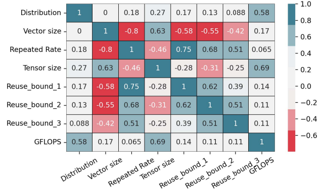
Fig. 5: Heatmap of the Spearman correlation coefficients. The correlation coefficients are among data characteristics ( Data Distribution , Vector Size , Repeat Rate , and Tensor Size ), three reuse bounds, and GFLOPS.
