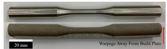
Figure 5: Conventionally machined (top) and as-built LPBF fatigue samples before any post processing. Slight warpage of AM sample is realized in the direction away from the attached support structure.
