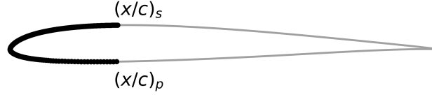
Fig. 2 Schematic showing limits of integration for calculating BEF and LESP . x/c for BEF is set to 0.01c based on prior results [3]; x/c for LESP is set to location of maximum airfoil thickness [2].
