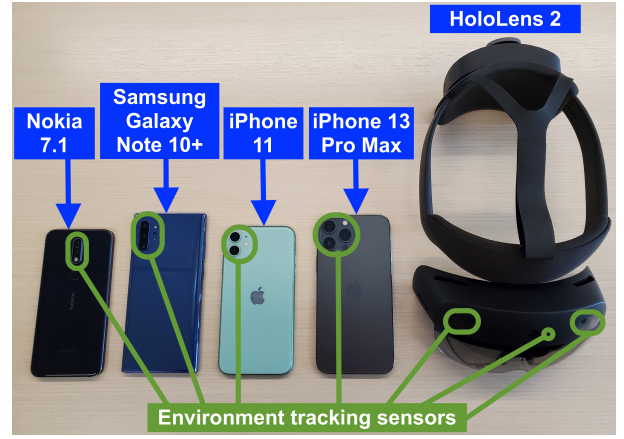
Fig. 4: The AR devices used in our experiments. On the HoloLens 2 tracking cameras are spaced farther apart, with the depth sensor just off-center.
