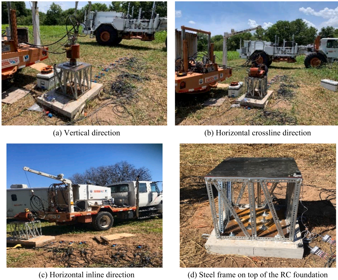
Fig. 3. Orientation of the shaker (Thumper) installed on top of the steel frame.
