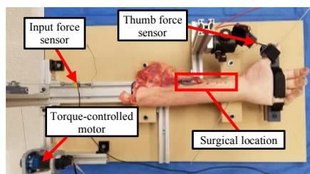
Figure 2. Custom testbed setup used to measure key pinch force in a human cadaver forearm.
