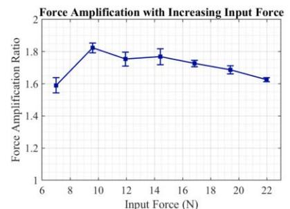
Figure 3. Force amplification ratio created by the implant-based tendon transfer surgery with increasing input force (n = 1).
