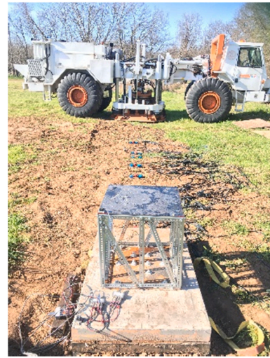
Fig. 4. Typical passive isolation test setup.
