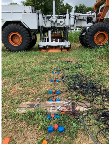
Fig. 2. Installed barrier and mobile shaker truck.
