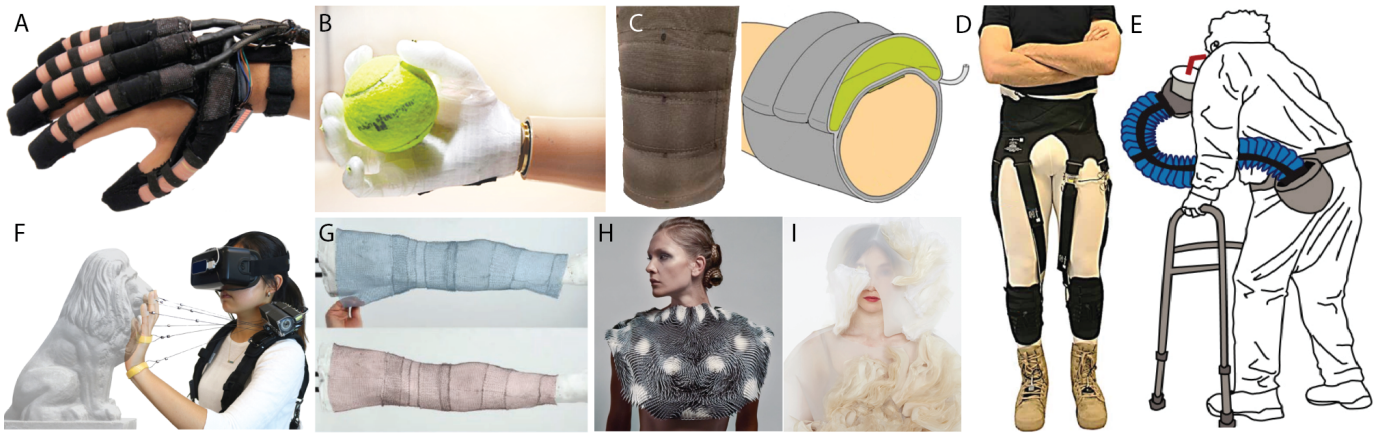
Fig. 1. Examples of soft wearable devices in diverse application areas. A. Pneumatic glove for hand rehabilitation [13]. B. Cable-driven soft prosthetic hand [21]. C. Segmented pneumatic actuation for compression therapies [7]. D. A cable-driven suit for reducing metabolic costs of walking [9]. E. A supernumerary pneumatic arm for aiding activities of daily living [11]. F. A string-based wearable haptic interface for virtual reality [22]. G. Leggings knitted from shape memory alloy (SMA) that can contract to match the limb shape [23]. H. An expressive soft robotic garment actuated by SMAs responds to the gaze of others [24]. I. A piezoelectric garment reacts to ambient illumination [25].
