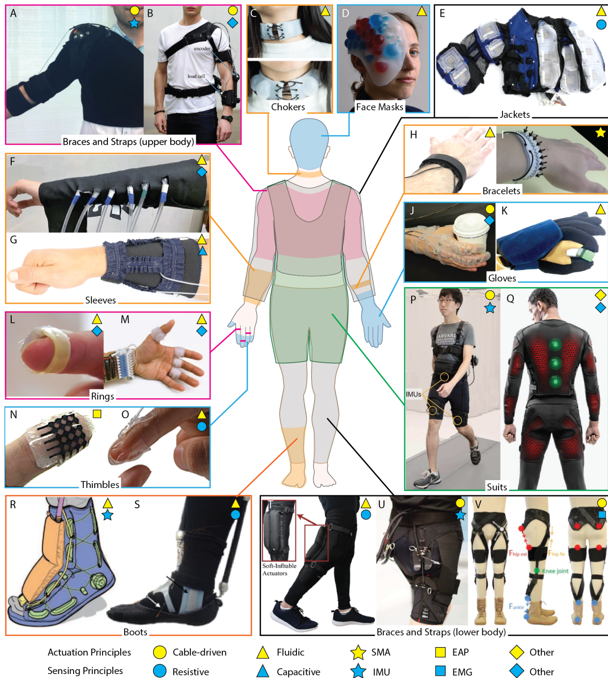
Fig. 2. Examples of soft wearable robotics and haptic devices in various wearable form factors. Yellow and blue symbols represent different actuation and sensing principles respectively. A-B. Devices consist of braces and straps on the upper body [18], [51]. C. Biometric chokers [52]. D. Responsive face prosthesis [53]. E. Haptic jackets [54]. F-G. Sleeves [48], [55]. H-I. Bracelets [56], [57]. J-K. Gloves [16], [58]. L-M. Rings on different segments of fingers [17], [36]. N-O. Thimbles [59], [60]. P-Q. Suits [10], [61]. R-S. Boots [19], [62]. T-V. Braces and straps for lower body [9], [20], [63].
