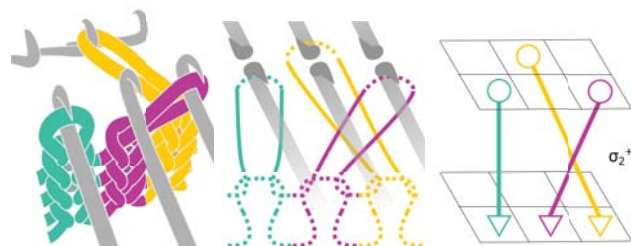
Fig. 1: The arrangement of loops on a knitting machine (left) can be represented as a braid (right) by ordering the needles and collapsing each loop into a single strand.
