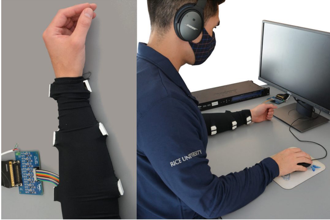
Fig. 1. Participant wearing the vibrotactile sleeve, positioned to complete the experimental task. (left) Vibrotactile sleeve used in experiments to deliver vibrotactile cues to the participant via 6 vibrotactors. Tactors were evenly spaced on the participant's forearm between their wrist and elbow with 3 vibrotactors on the ventral side of the arm and 3 vibrotactors on the dorsal side. (right) Participant wearing the vibrotactile sleeve while interacting with the experimental GUI on the monitor and listening to pink noise through headphones. (Color figure online)
