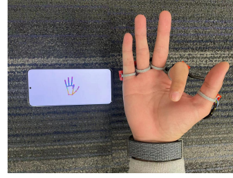
(b) Wireless streaming of sensor data to mobile device which performs 3D finger motion tracking
