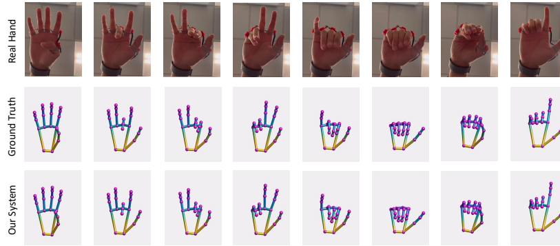
Fig. 2. Comparison of 3D finger tracking results between ground truth and ssLOTR
