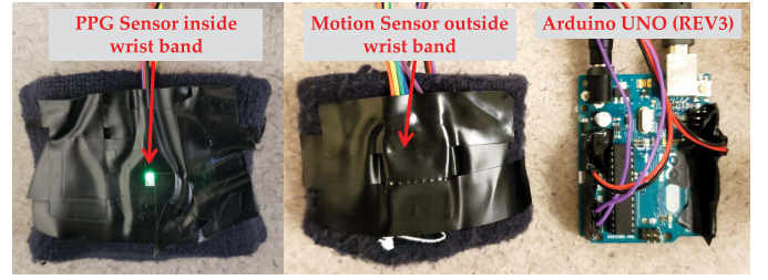
Fig. 7. Prototype: wrist-worn PPG sensing platform.
