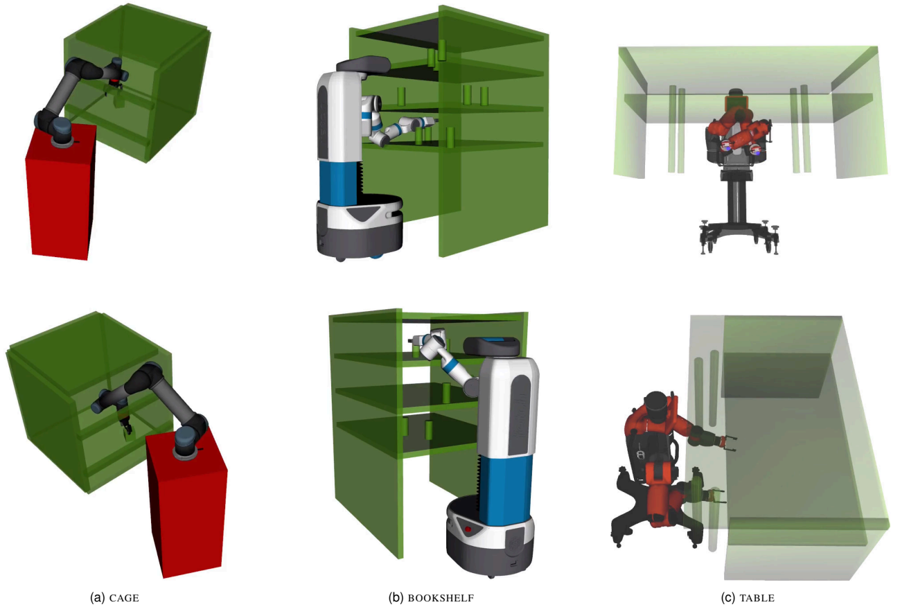
Figure 3: Samples of problem instances used in our experiments. The positions and orientations of the objects in the scene are randomized relative to the robot. The start configurations are uniformly sampled from the robot’s collision-free C -space. The goal configurations are randomly selected according to the problem. For illustration purposes, we show only the goal configurations. (a) CAGE problem: a UR5 (6-DOF) robot reaches for a box inside a constrained cage. (b) BOOKSHELF problem: a Fetch (8-DOF) robot reaches deep inside a bookshelf to pick the cylinder at the back. (c) TABLE problem: a Baxter (14-DOF) robot tucks both its arms between the bars under the table, given a small space allowance. In some problem instances, the arms need to be tucked crossed (top).
