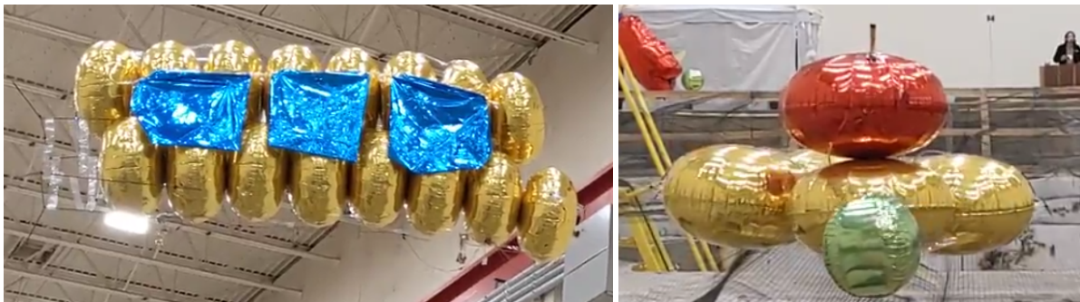
Fig. 10 Left: "caterpillar" blimp design to achieve on-board ball tracking. Right: "crab" blimp design to scoop game balls off the net-covered pit.
